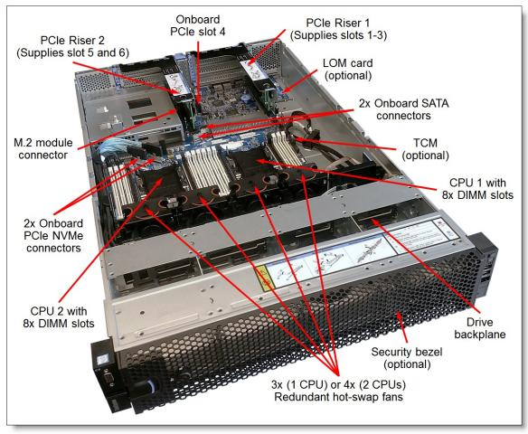
The following figure shows the locations of key components inside the SR590 server.
