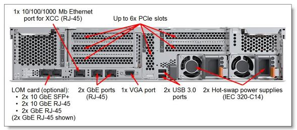
Figure 5. Rear view of the SR590
