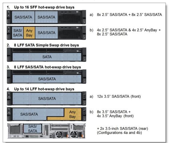
Figure 7. Internal drive bay configurations
